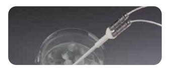
Field-proven method of determination: Put the temperature probe in an ice cold water bath and let it reach a steady-state. Then transfer it quickly to a column of steam and monitor its resistance until a steady state is reached again.
