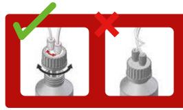
The special feature: The body of the distributor can be turned independently from the screw cap. This means, that the completely assembled distributor can be removed and fixed on another bottle without the risk of disarranging the tubing.
