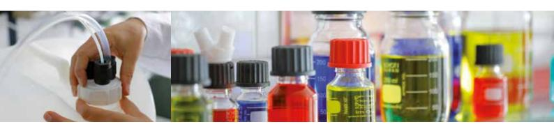
All fluoroplastics, PTFE, PFA and FEP have a smooth, non-wetting surface and can usually be cleaned without any problems. Abrasive scouring agents might damage the surface and result in a milkiness of the vessels – especially those made of PFA and FEP. You may use all neutral detergents (pH 7). For a stronger contamination we recommend to use an alkaline detergent up to pH 12. Clean or dry vessels in a laboratory washing machine only when they are completely opened.
